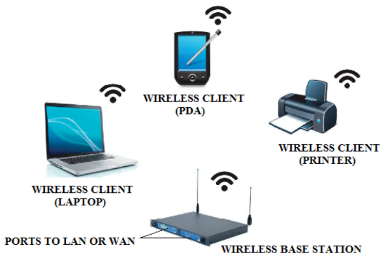
Figure 4.1. A simple wireless network
